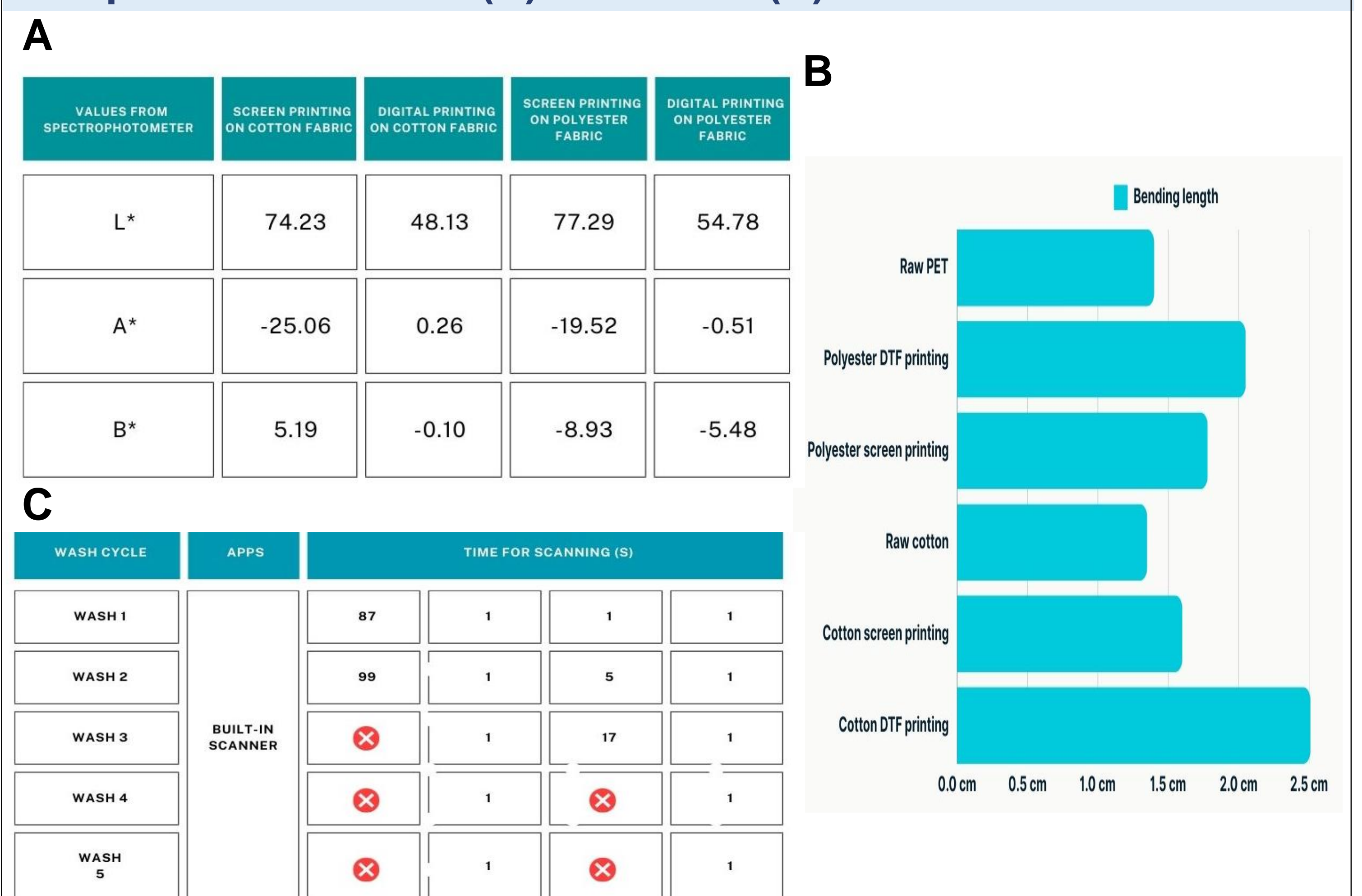
Figure 3: Data Color Values of Printed Fabrics (A), Bending Test Results (B), and Scanning Performance after 5 Wash Cycle (C)
