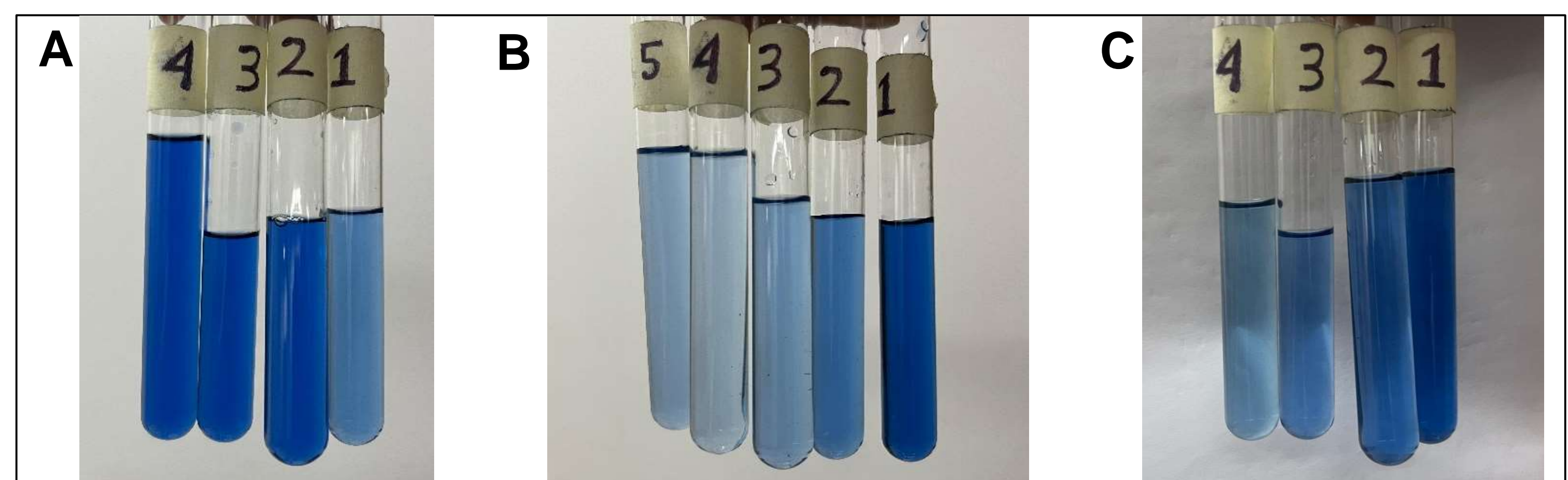
Figure 5: Dye Solution Before and After Batch Adsorption Experiment (A) pH (B) Biomass Dosing & (C) Contact Time Variation
